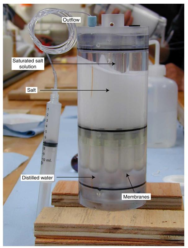
**Figure F3.** Photograph of an osmotic pump and several Teflon sampling coils being filled with distilled water by a peristaltic pump.
