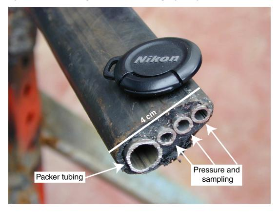
Figure F14. Umbilical for packer inflation and sampling tubing.
