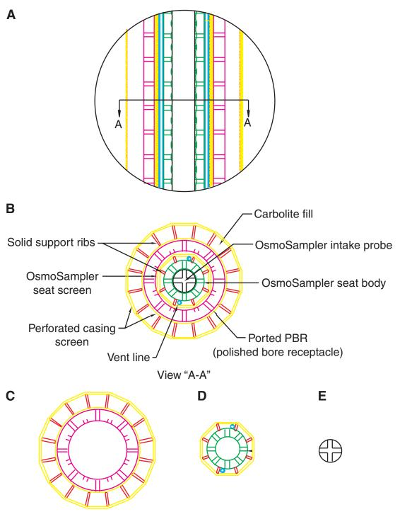
**Figure F7.** Schematic of an OsmoFlowmeter. Tracer fluid is injected at the center of the sampling volume at a constant rate that mixes with the naturally flowing pore fluids. The mixed fluid is continuously sampled at the four sampling ports. The varying amounts of tracer within these samples will be used to determine flow rate and relative direction.
