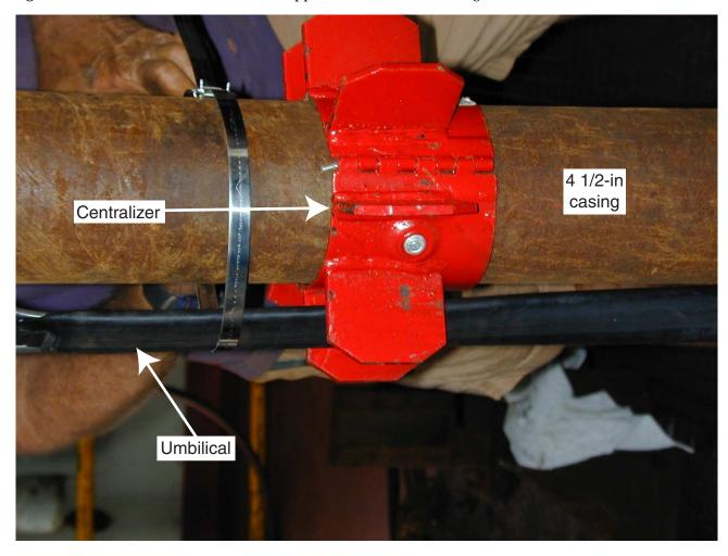
Figure F15. Centralizer and umbilical strapped onto the 4½-in casing.
