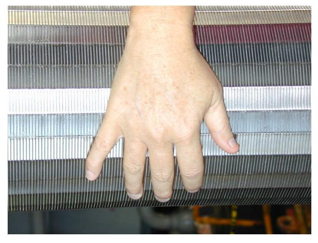
Figure F13. Close-up photograph of the wrapped screen.
