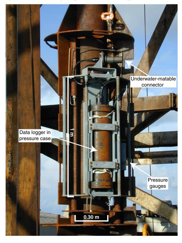
Figure F11. CORK-II head bay with pressure sensor and data logger.
