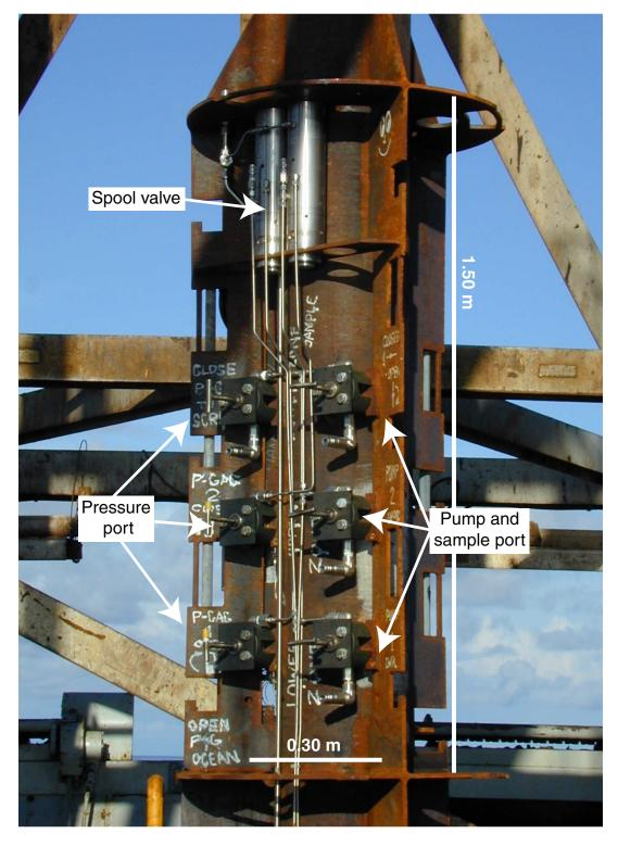
**Figure F21.** Hole 1253A CORK-II OsmoSampler installation space-out. mbsl = meters below sea level, mbrf = meters below rig floor, mbsf = meters below seafloor.
