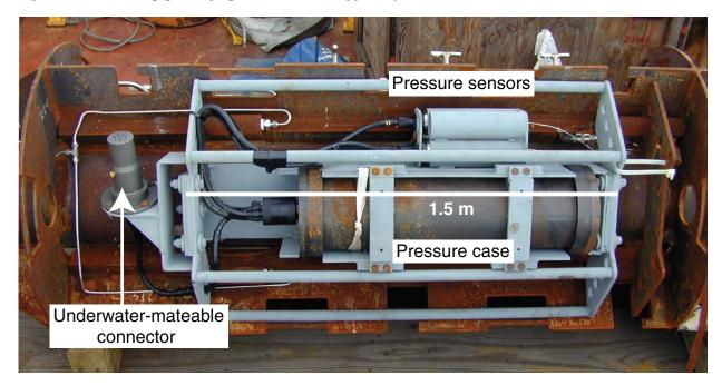
**Figure F10.** Close-up photograph of the data logger bay of the CORK-II head.
