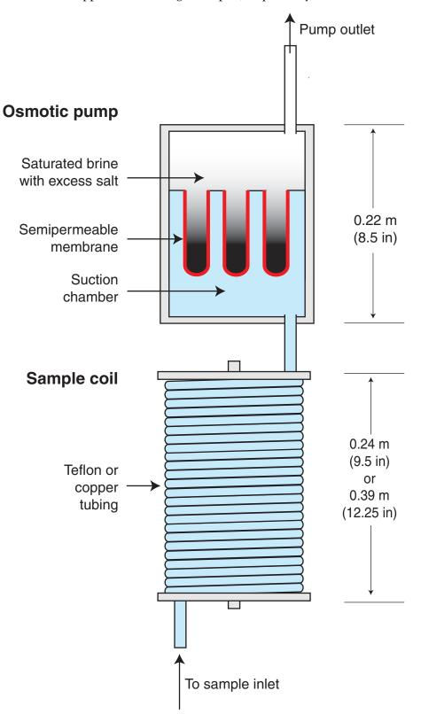
**Figure F2.** Photograph of an osmotic pump. The excess salt slowly dissolves throughout the experiment to keep the solution within the upper chamber saturated as brine is expelled through the outflow.
