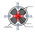
**F8**. Intake configuration for Osmo-Sampler and OsmoFlowmeter, p. 22.
