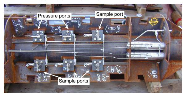
Figure F17. Close-up photograph of the plumbing and valve bay of the CORK-II head.
