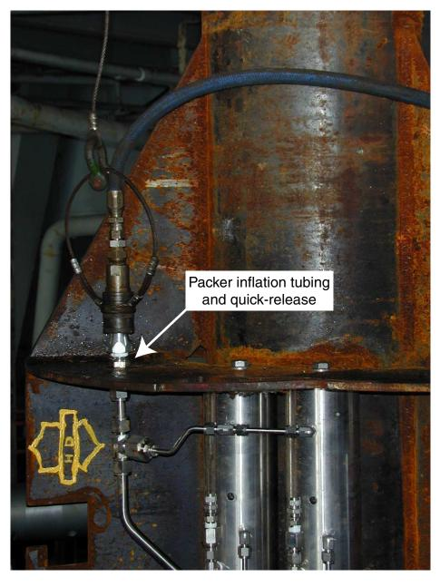
Figure F18. Packer inflation tubing and quick release.
