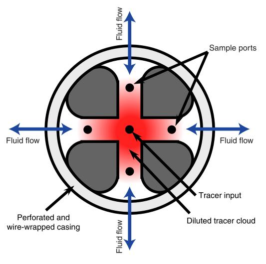
**Figure F8.** Intake configuration for OsmoSampler and OsmoFlowmeter in the sampling probe from Hole 1255A.
