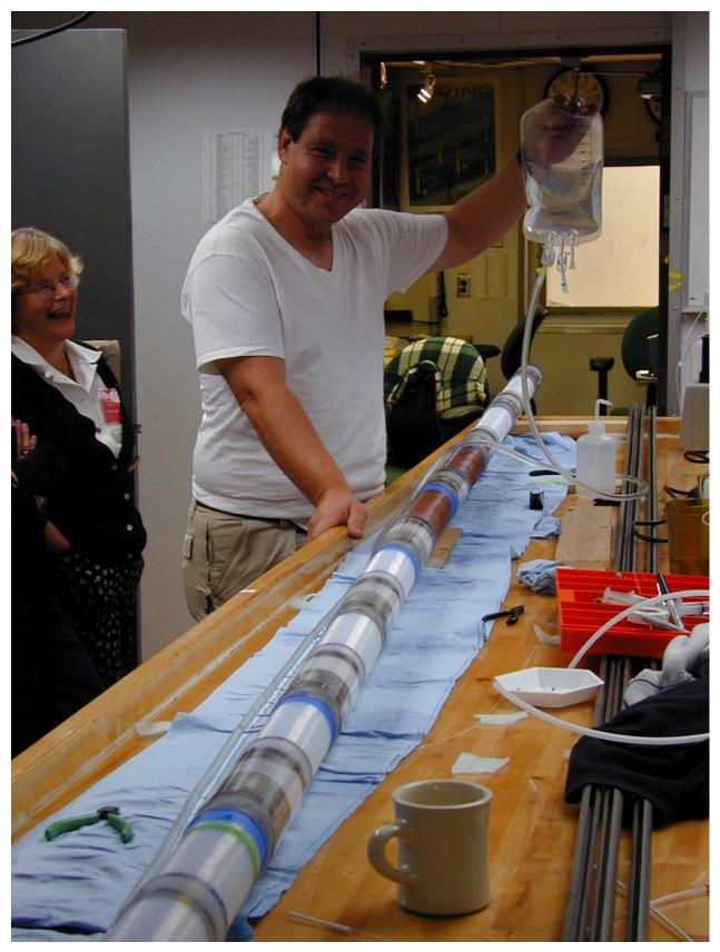
Figure F5. Assembly of an OsmoSampler package. (J. Morris, left, and H. Jannasch, right, are also pictured.)
