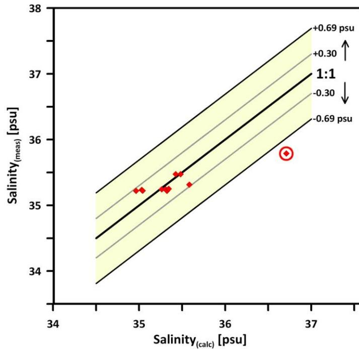
**Figure S3: Measured vs. reconstructed Salinity.** Calculated salinity values (red dots) fall within  $\pm 0.30$  psu of the measured core top values except for one outlier. Estimated standard deviations [Schmidt, 1999] at  $\pm 0.69$  and  $\pm 0.30$  psu are shown in black and grey respectively.
