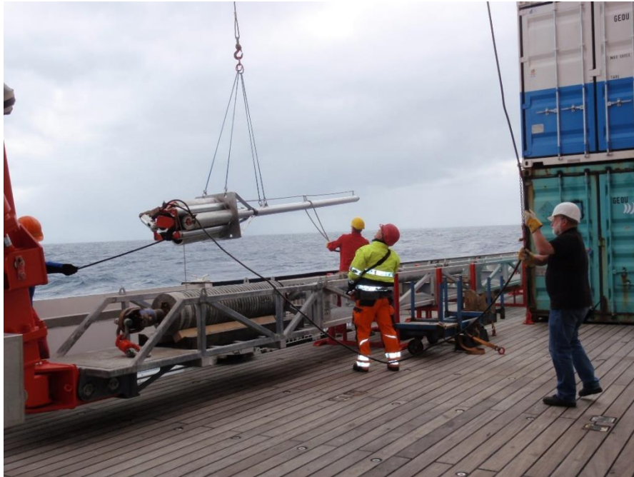
Fig. 5.3.1: Deployment of the Bremen heat probe during SO247.
