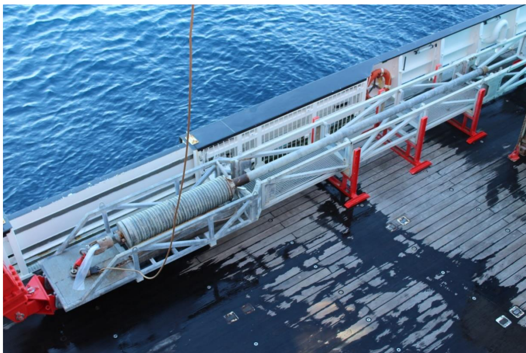
Fig. 5.4.1: Gravity corer within the cradle on board SO247.
