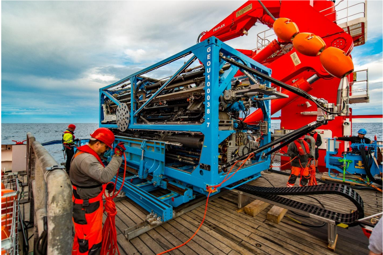
Fig. 5.4.2: The sea floor drill rig MeBo200 on DSRV SONNE.
