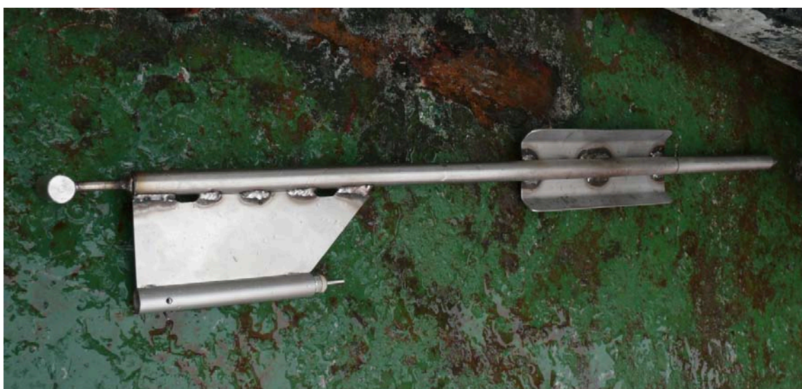
Figure 32: MTL stick to be deployed by ROV; those systems complement the MeBoPlugs at two sites to get high-resolution seafloor temperature variations as reference for the MeBoPlug data. ROV handle is seen left, MTL is hosted in a metal tube; lower portion is stuck into the sediment (with metal shield for stabilisation in case of bottom currents).
