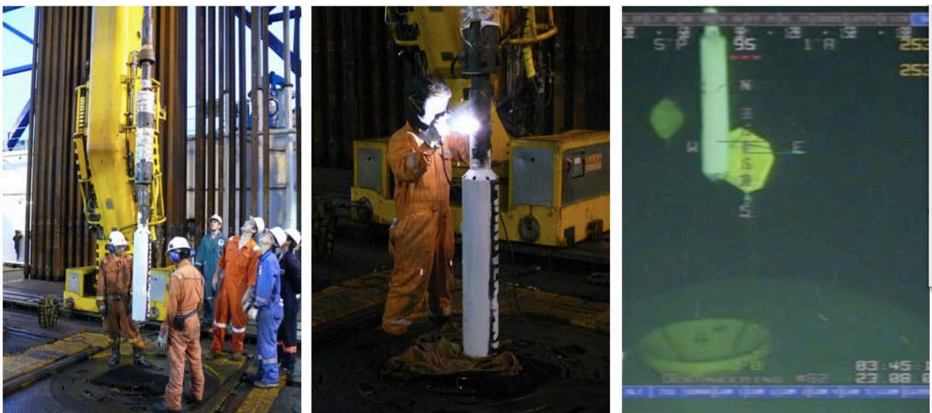
Figure 8: “Mini-CORK” observatory consisting of a retrievable Bridge Plug to separate the borehole from the overlying ocean water hydraulically (left, top), and a pore pressure instrument attached to bridge plug (left), additionally secured by tack-welding (middle), and at the drill string in appx. 2500 m waterdepth prior to re-entry of hole C0010A (right).
