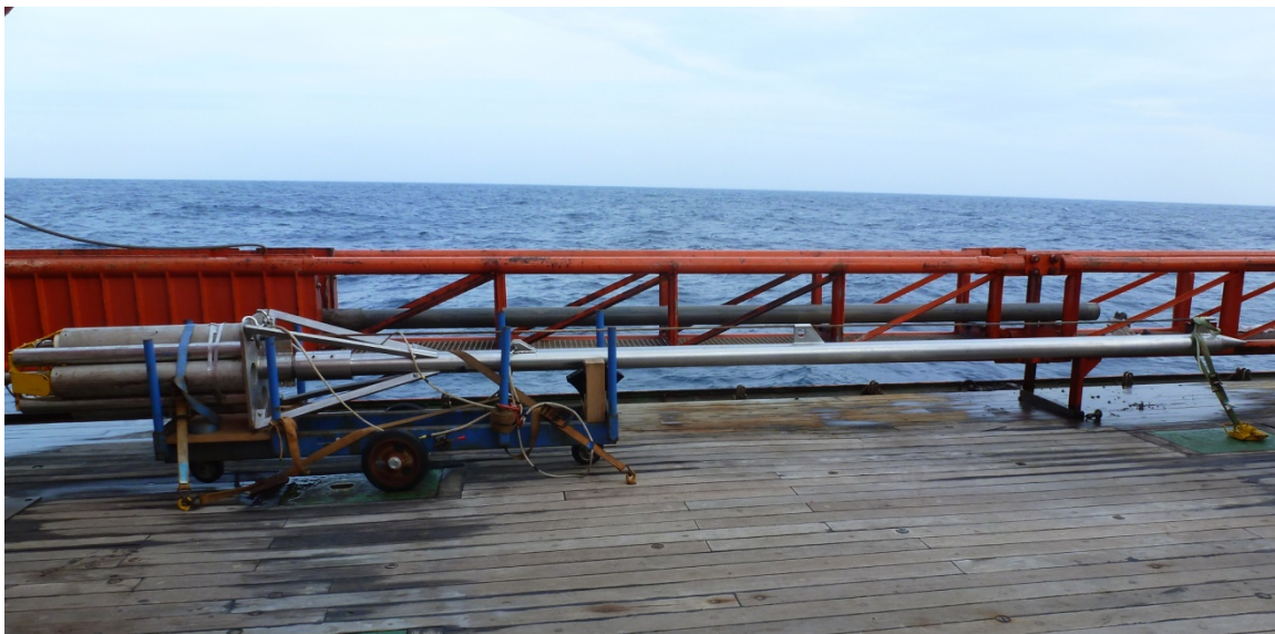
Figure 11: The 6 m-long Bremen heat flow probe on the working deck of R/V Sonne .
