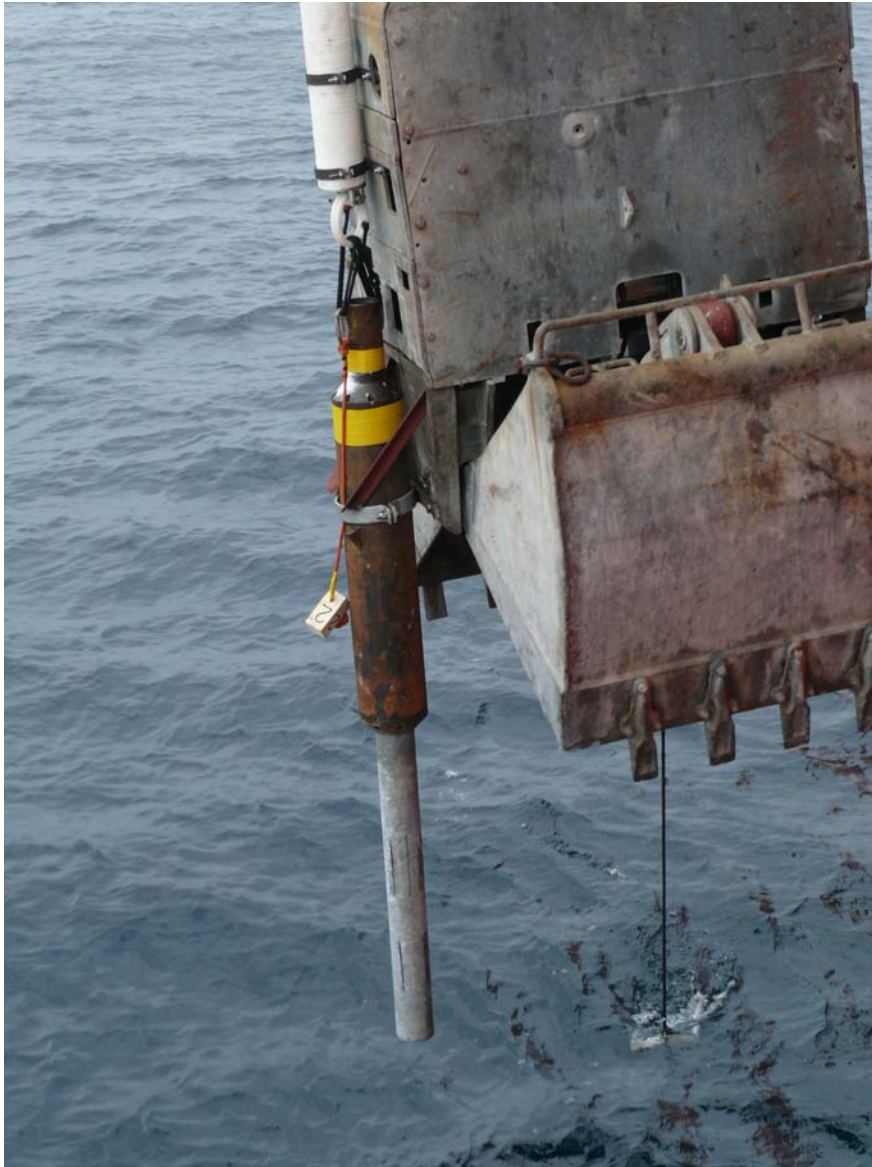
Figure 64: SmartPlug piezometer mounted to releaser and TV-grab when going overboard on MV#4.
