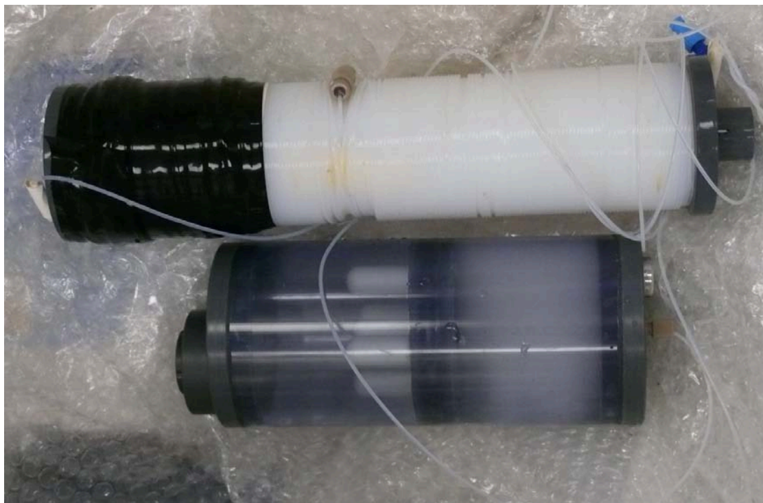
Figure 30: Osmo-sampler (tubing coil [top] and pumps [below]) that are hosted in a PVC tube attached to MeBoCORK B.
