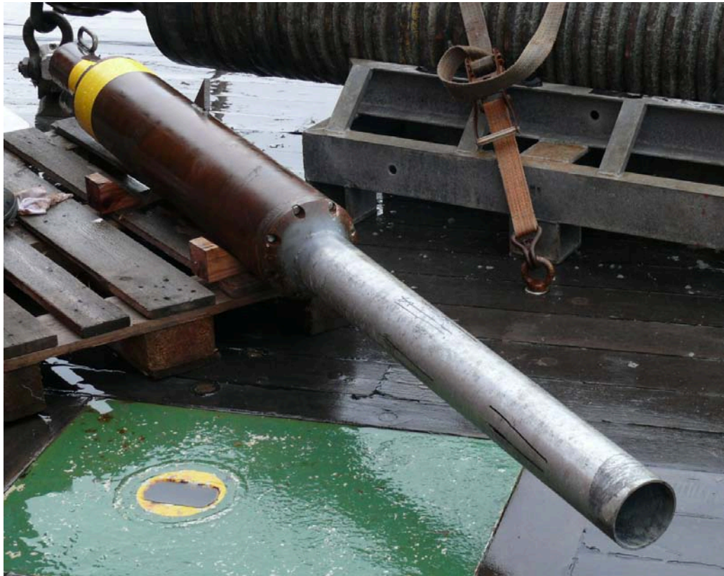
Figure 33: SmartPlug converted into a piezometer before being mounted to the TV-grab for deployment.
