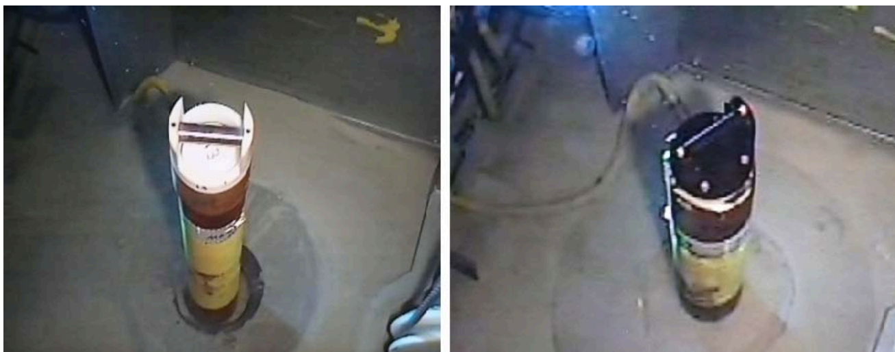
Figure 61: MeBoPlug (left) and MeBoCORK B top hole assembly with black endcap (right) after installation with MeBo. Photos were taken immediately before the seafloor drill rig takes off the ground. See text.
