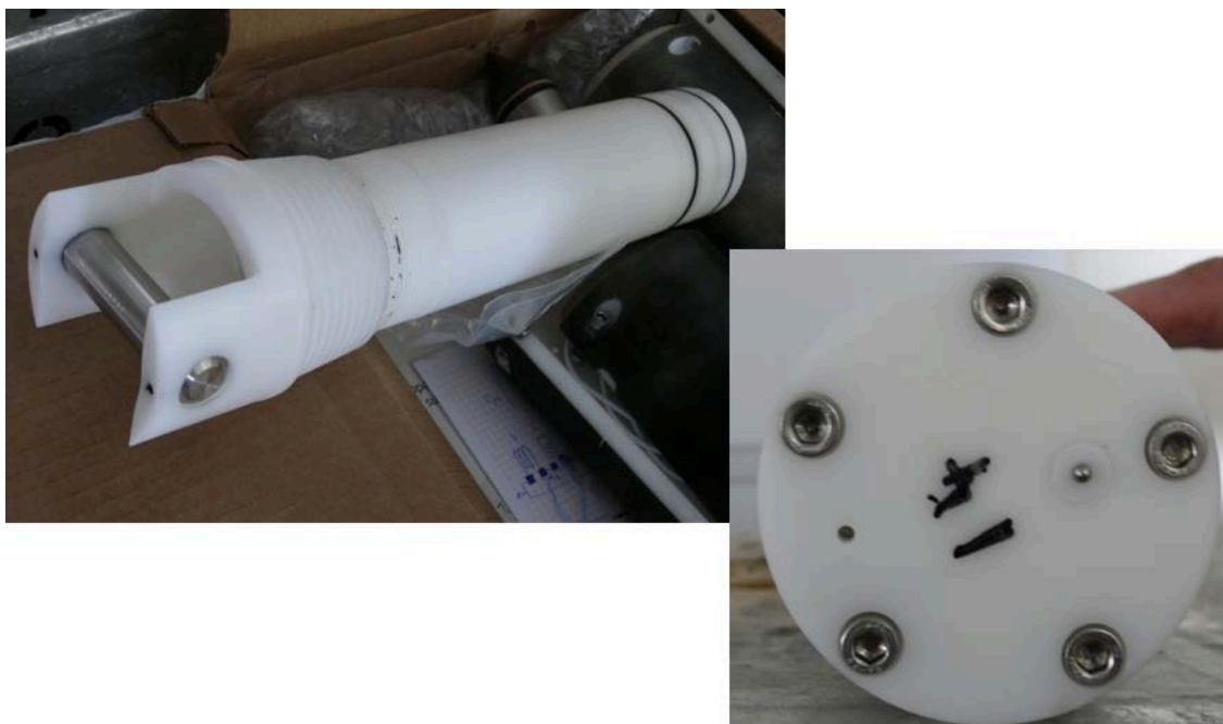
Figure 31: MeBoPlug prior to being screwed into a MeBo drill pipe (left); right photograph shows bottom view into the borehole with ports for P [hole at left] and T [little pin at right] monitoring. See text.
