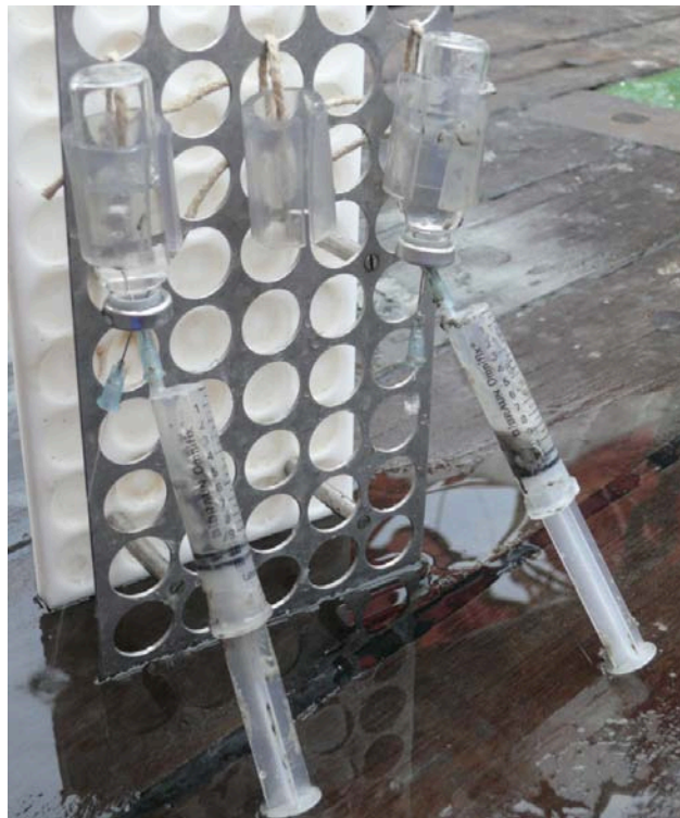
Figure 24: Gas hydrate samples from gravity cores were transferred into syringes for dissociation; free gas is ascending into vials for later laboratory analysis..
