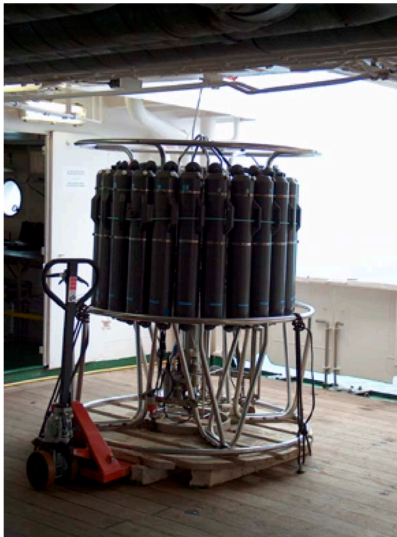
Figure 10: CTD on main deck of RV Sonne prior to deployment.
