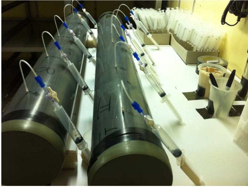
Figure 25: Rhizon pore water extraction in split working half of the gravity core.
