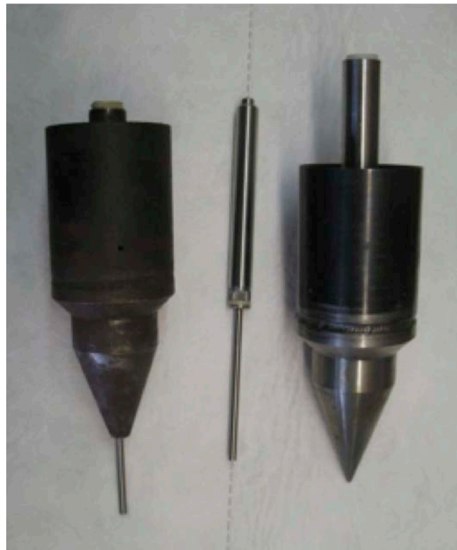
Figure 21: In situ temperature probes used during cruise SO222.
