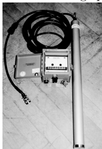
Figure A.3: Borehole Tiltmeter, AGI 722a, with connector and connection terminal.
