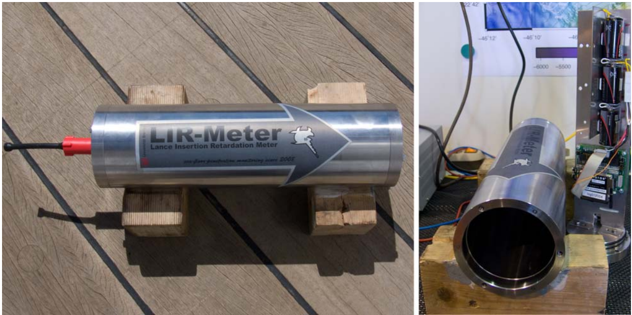
Fig. 5.12 Left: LIR-Meter in pressure casing; right: electronics
