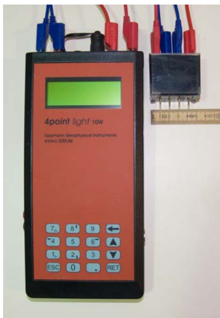
Fig. 5.11 4point-light geoelectric measurement system for measurements of electrical resistivities on split cores.
