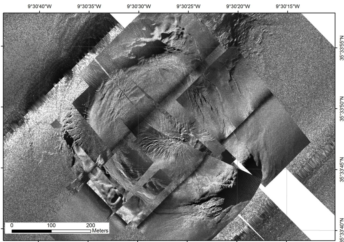
Fig. 4.2.2.13: Sidescan sonar processed mosaic of Porto mud volcano, acquired at both low and high resolution (120kHz, 410kHz). The top displays an asymmetric pattern of flows, it is also clear the network of incised channels in the sides and some areas with different textures near the foot of the slope of this edifice.
