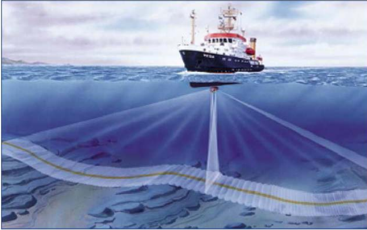
Fig. 4.1.1: Basic principle of a multibeam echosounder
