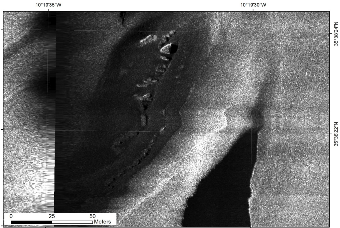
Fig. 4.2.2.14: Rock outcrops imaged from the west, acquisition at 120kHz.
