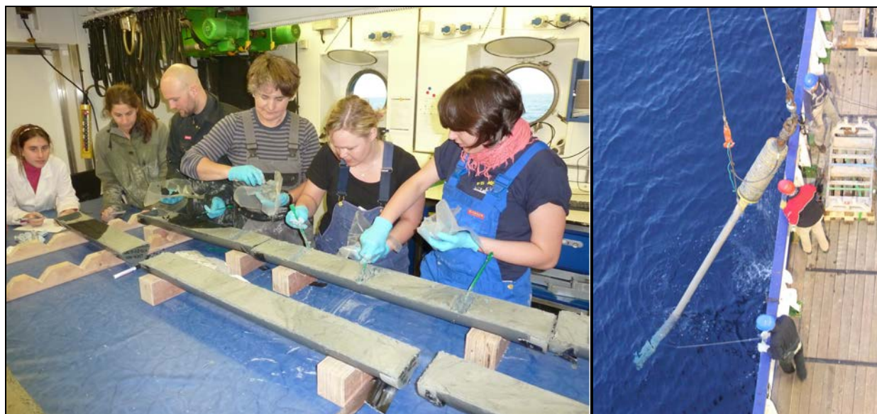
Fig. 4.4.2: Gravity corer retrieval and sampling.
