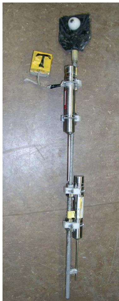
Fig. 2. Mini-temperature lance equipped with two MICREL THP temperature sensors.
