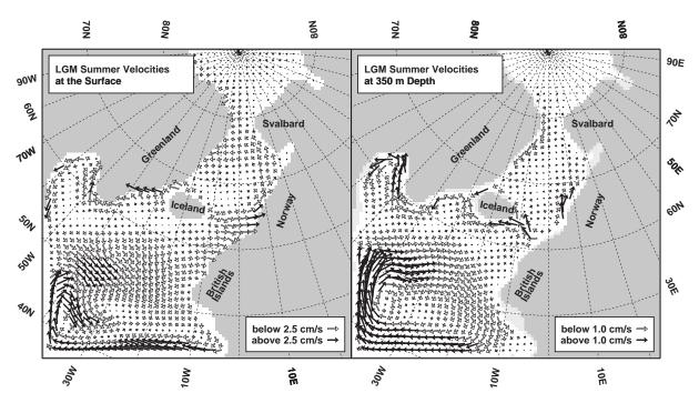
Figure 4: Modelled glacial summer circulation at the surface (left) and 350 m depth (right). Only one vector in two is displayed for clarity. The currents, especially the flows into and out of the GIN Seas, are quite similar to modern conditions.
