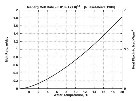
Figure 2: Iceberg decay as function of water temperature, after laboratory experiments by Russel-Head (1980).
