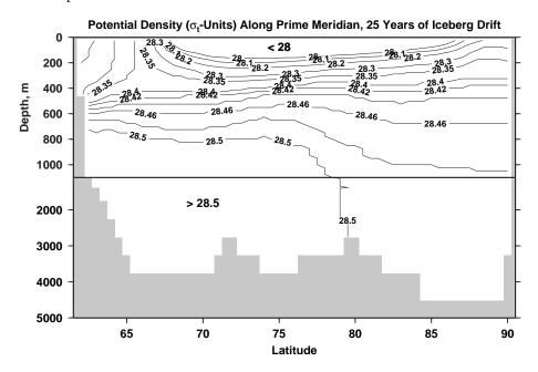
Figure 8: Meridional potential density section along Prime Meridian for the iceberg experiment. The melting icebergs impose a lid of relatively fresh water over the GIN Seas and stop the convection there. Contour interval:  $0.02 \text{ g/cm}^3$ .
