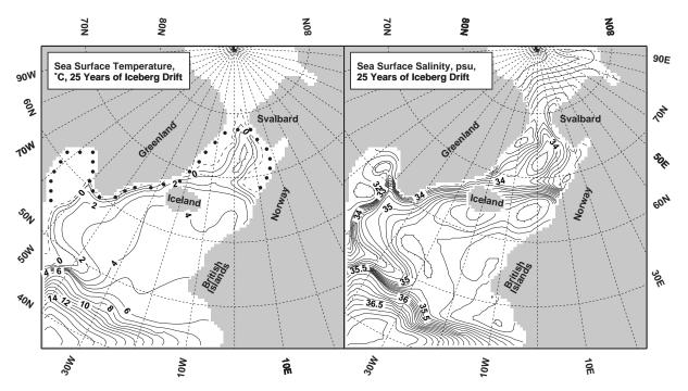
Figure 6: After 25 years of integration with icebergs, both sea surface temperature (left) and salinity (right) are greatly reduced all over the Greenland, Norwegian, and Labrador Seas, and a cold and fresh tongue extends towards Europe along 50 N. Contour intervals: 1 °C, 1 psu below 33, 0.2 psu between 33 and 35, and 0.1 psu above 35 psu. Dots indicate iceberg generation locations.
