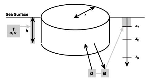
Figure 1: In the model, icebergs are represented by idealized pie-shaped blocks of ice. Explanation of symbols: T = water temperature, u, v = horizontal velocities, h, r = iceberg height and radius, Q = heat flowing from water into ice, M = meltwater runoff from iceberg to water, and  $z_{1...3} = depths$  of model layer interfaces.
