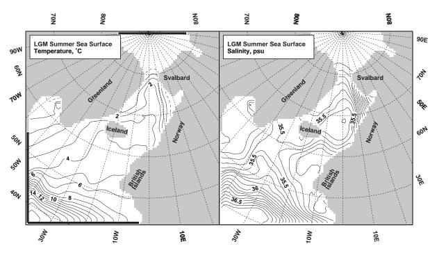
Figure 3: Sea surface temperature (left) and salinity (right) for the glacial summer, reconstructed from sediment-core based temperature estimates and oxygen isotope measurements (Schäfer-Neth, 1994, 1998). The coastline differs from the modern due to the lower glacial sea level. Contour intervals: 1 °C and 0.1 psu. Heavy black lines along the southwestern and northern boundaries indicate restoring zones.
