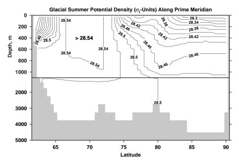
Figure 5: Meridional section of potential density along Prime Meridian for the glacial reconstruction. At about 69 N, there is a chimney of dense water with  $\sigma_t \geq 28.54$  gcm<sup>-3</sup> extending from the surface down to 1200 m. In resemblance to modern conditions, this gives clear evidence of deep convection. Contour interval: 0.02 g/cm<sup>3</sup>.
